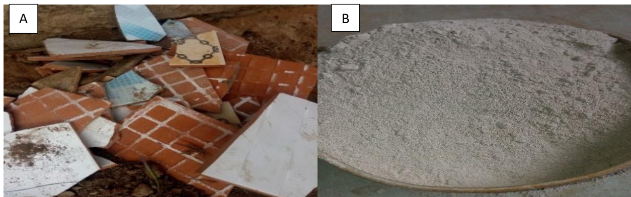
Plate 1: A: Ceramic Tiles Waste from Demolition Site and B: CTWD after Grinding
