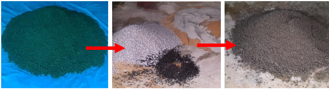
Plate 1: Material for Crumb-Rubber Masonry Concrete
